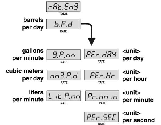
To select a unit of measure for rate, press **INCREMENT** until the desired unit of measure appears in the bottom display. If you selected a user-defined unit of measure for volume in Step 2, your rate unit options will be per day, per hour, per minute, or per second.
