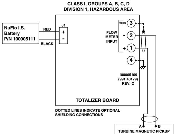
TURBINE MAGNETIC PICKUP MAY BE 991 OR 458 SERIES NUFLO FLOWMETER OR ANY APPROVED DEVICE WITH THE FOLLOWING MAXIMUM ENTITY PARAMETERS:
